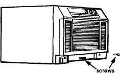
**13** Attach front by first <u>removing</u> the two, #8 x 9.5mm (3/8") screws from base; then insert front tabs into top of cabinet and swing front in place. Attach bottom of front by reinserting the two screws.
